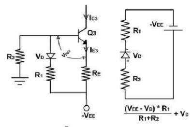
$$(V_{EE} \cdot V_D) = \frac{R_1}{R_1 + R_2} + V_D = V_{BE3} + I_{E3}R_E$$
